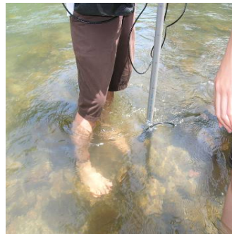
Figure 13 : Flo-Mate Model 2000 Portable Flow meter and Velocity measurement procedures
