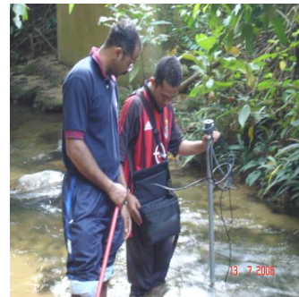
Figure 13 : Flo-Mate Model 2000 Portable Flow meter and Velocity measurement procedures
